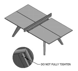
WITH HELP, LIFT THE "MOVING" TOP INTO POSITION JUST AS IN THE LAST STEP AND SLIDE IT TOWARD THE TABLE UNTIL IT COMES IN CONTACT WITH THE BLADE. USE 4 OF THE 4" BOLTS TO VERY LOOSELY FASTEN THE BATTENS TO THE BEAMS. DO NOT FULLY TIGHTEN THE NUTS. THE MOVING TOP NEEDS TO BE ABLE TO SLIDE BETWEEN AN OPEN AND CLOSED POSITION TO ACCEPT THE BLADE (NET)
