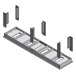
2 IDENTIFY THE PAIRED END LEGS (LEFTS AND RIGHTS) AND CENTER LEGS. THEY WILL BE INSTALLED ON THE TABLE AS SHOWN.
