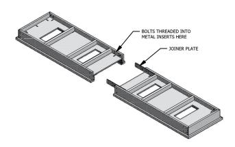
PLACE THE CRADLE HALVES IN POSITION IN YOUR ROOM AND LAY THEM UPSIDE-DOWN ON A PROTECTIVE SURFACE SO THAT NO DAMAGE IS DONE TO YOUR FLOOR OR TO THE CRADLE. FASTEN THE TWO HALVES TOGETHER USING THE JOINER PLATE AND THE BOLTS PROVIDED.
