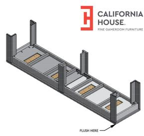
PLACE THE LEGS IN POSITION AND FASTEN THE LEGS TO THE CRADLE USING THE BOLTS PROVIDED. BEFORE TIGHTENING THE BOLTS, ADJUST THE POSITION OF THE END LEGS SO THAT THEY ARE FLUSH WITH THE END OF THE TABLE TOP RAIL.
