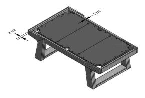
AFTER APPLYING COVER TO THE RAIL FRAME, LIFT IT IN PLACE ON THE TABLE. CENTER THE RAIL FRAME ON THE CHASIS AND LEGS. USE THE SCREWS YOU REMOVED IN THE FIRST STEP TO FASTEN THE RAIL FRAME TO THE CHASIS. WHEN IT IS FASTENED FIRMLY IN PLACE, USE THE 1 3/4" BOLTS WITH COMPRESSION WASHERS TO FURTHER FASTEN THE RAIL FRAME TO THE SLATE.
